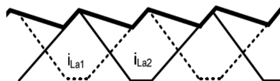
Fig.9. Interleaving between two input inductor currents.
