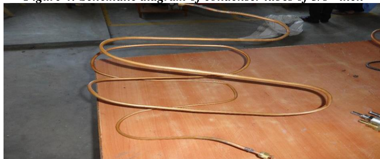
Figure 5: Schematic diagram of condenser tubes of 3/8^{\text{th}} inch
