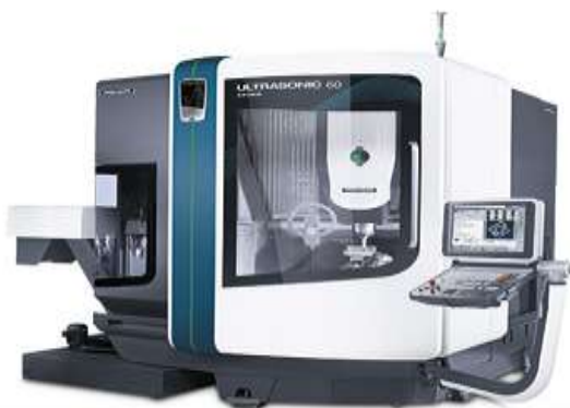
Figure 2: 5-axis Rotary Ultrasonic 60 Sauer Machine
