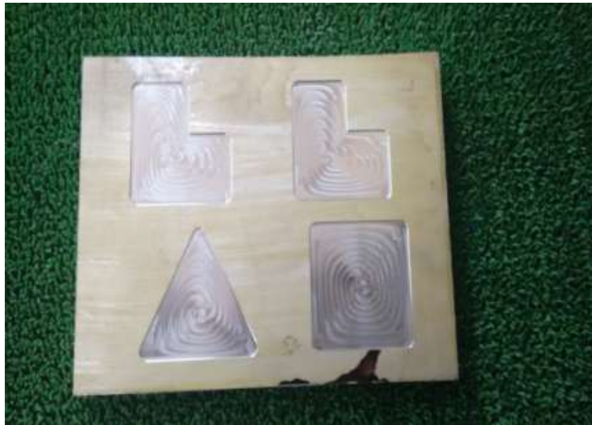
Figure 7: Pockets Machined Using Generated Tool Path
