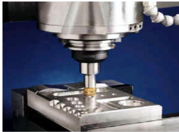
Fig. 1 End Milling Operation On AISI D2 Steel
