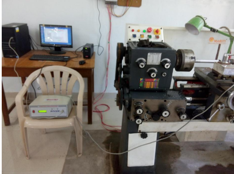
Figure.4 Shows tool dynamometer set up
