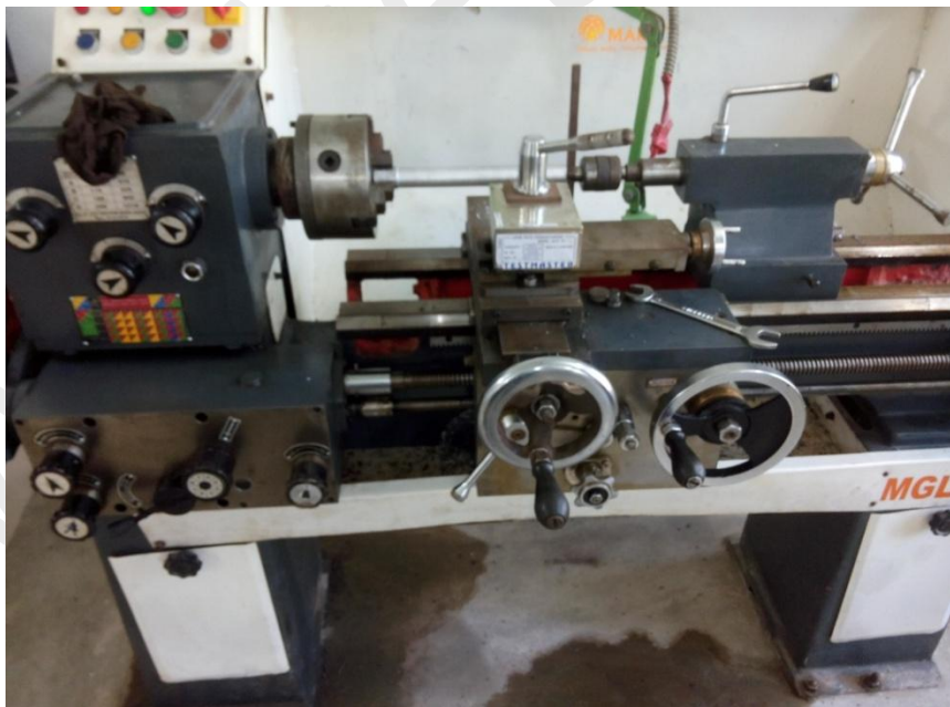
Figure.3 Shows High Speed Lathe Machine (MGL-54)
