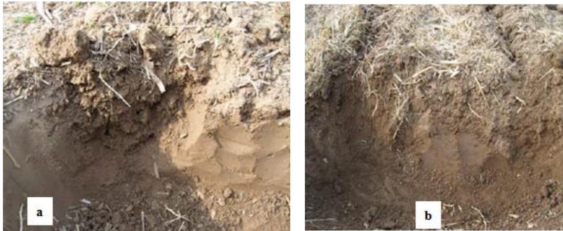
Fig. 7 (a) soil profile in vibrating shank. (b) Soil profile in no-vibrating shank.
