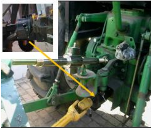
Fig. 2 Photographic view of PTO torque torsionmeter located between the tractor and the implement with a detailed view on the up-left photographic
