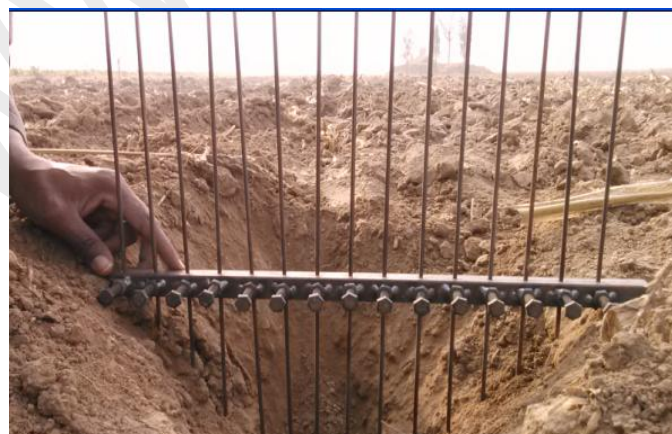
Fig. 4 Photographic view of Profilometer device used for measure soil profile
