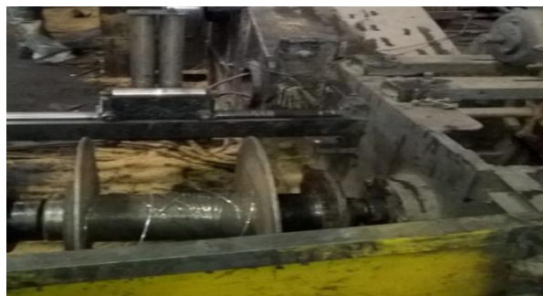
Figure.4-A Take Off Roller Of The Wire Drawing
