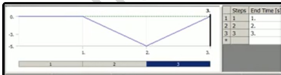
Fig. 3. Details of deformation applied in three load steps for analysis
