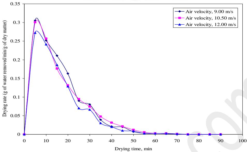
**Fig. 4: Effect of air velocity on drying rate of beetroots during drying at inlet air temperature 67.50 °C during FBD**
