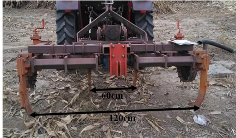
Fig. 1 Photographic view of new developed chisel plow.
