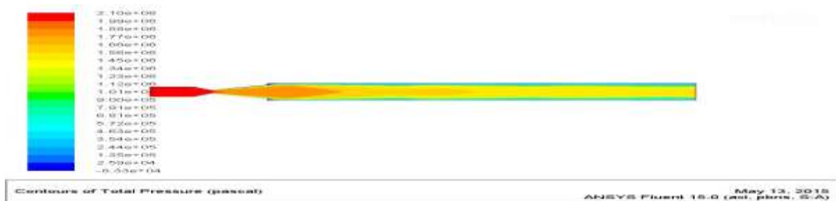
Fig.14 Pressure simulation of supersonic exhaust diffuser for length 1.4m with conical nozzle
